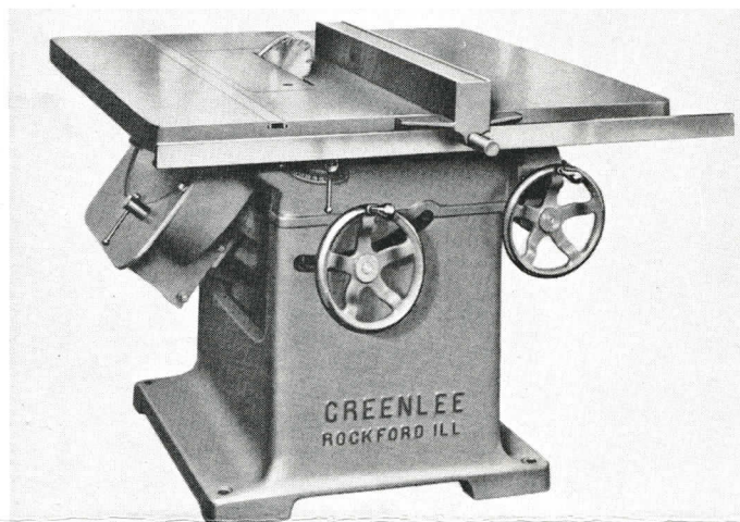
The double-faced, front-mounted ripping gauge shown above is optional on the 495, and recommended where set-ups require frequent changing from one side of the blade to the other.
