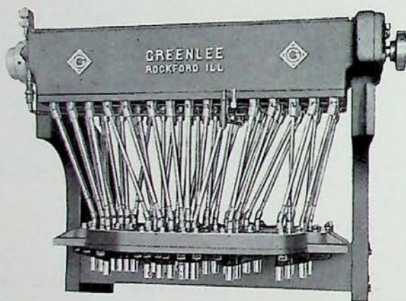
Upper Section of a Special 4-foot No. 386 Gang Borer equipped with 45 Universal Spindles for boring automobile body dash boards.
